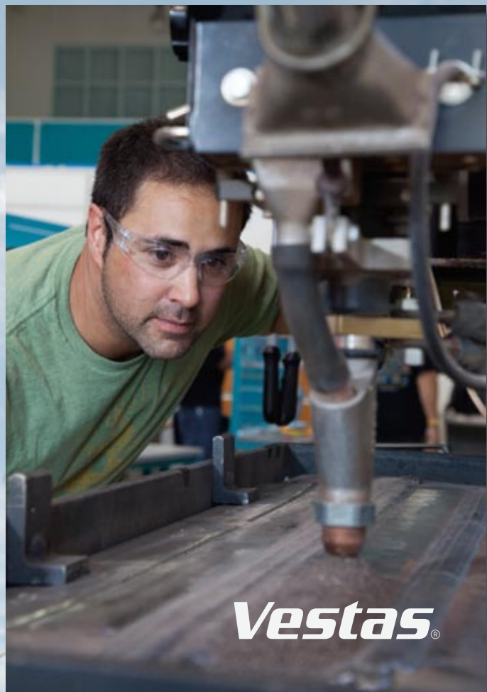
PCC's Economic & Workforce Development Division trains Vestas employees like Neil "Shane" Williams, pictured here preparing to use the sub-arc welding machine.
